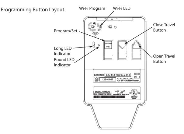
**NOTE**: Each programming step has a 30 second time limit for completion after the function is initiated. After 30 seconds, both LED's will illuminate RED indicating time has expired and the step must be restarted. Restart the step as many times as necessary to complete the programming.
